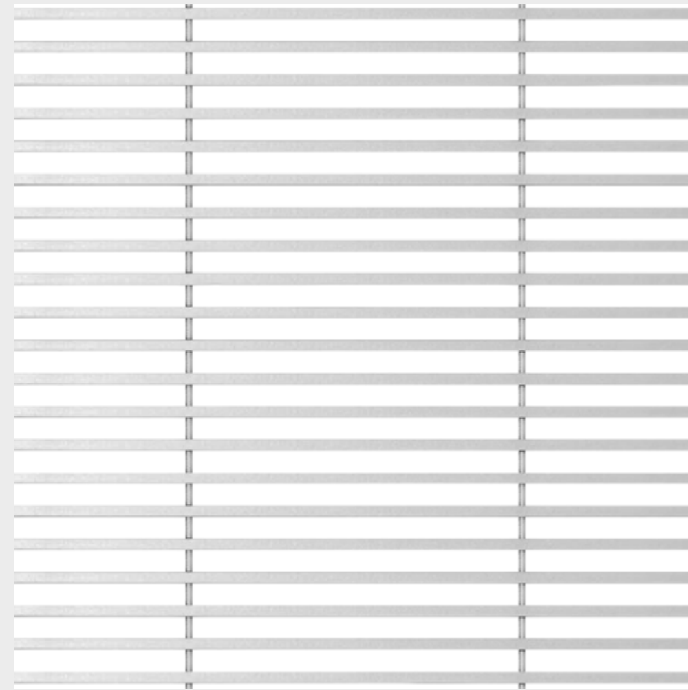
RADIUS Z07065 Open area: 65 % Material: SN Weight: 7,3 kg/m 2 Slot: 6,5 mm
