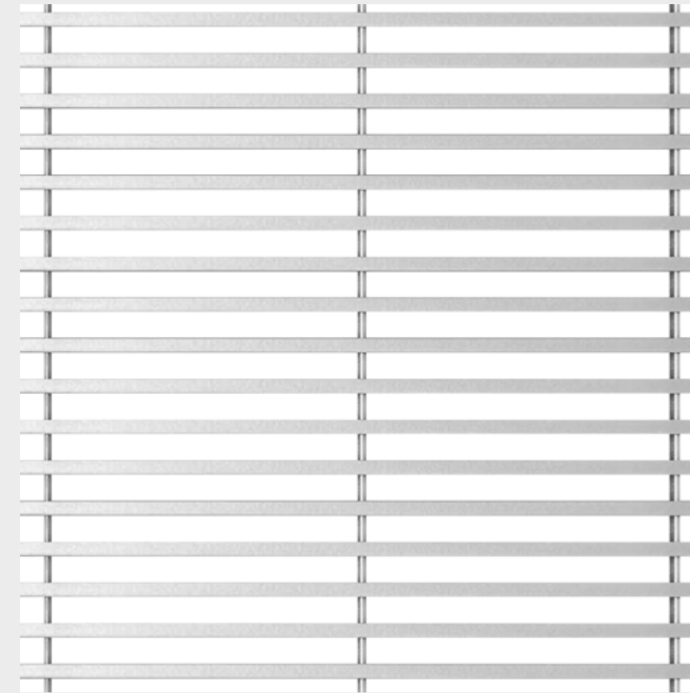
RADIUS Z10080 Open area: 65 % Material: PR Weight: 7,9 kg/m 2 Slot: 8,0 mm
